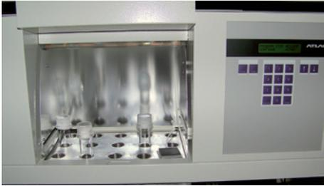
Figure 2: Standard irradiation laboratory system for determining photolysis of pesticides in aqueous solution
